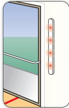
**Warning:** If mounting door monitor near metal frame, mount at least 8" away from metal frame.
