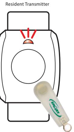
**B** Transmitter will blink 3 times to indicate transmitter has been activated.
