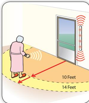
**Warning:** Door monitor will sound if door is opened and a resident wearing a transmitter is within 10-14 feet from door monitor. If the alert is triggered when a transmitter is too close or too far from door, or if you can pass thru door, call for technical assistance.
