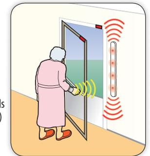
**Warning:** Door monitor will sound if door is opened and a resident wearing a transmitter is within 10-14 feet from door monitor. If the alert is triggered when a transmitter is too close or too far from door, or if you can pass thru door, call for technical assistance.
