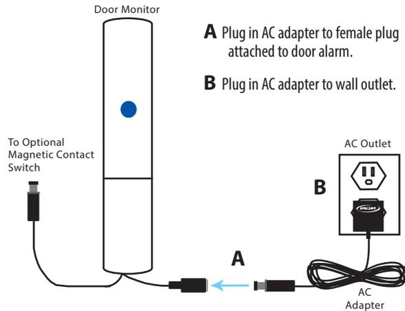
**A** Plug in AC adapter to female plug attached to door alarm.
