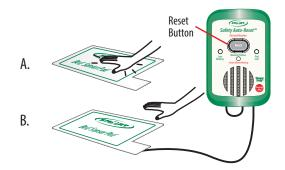
Test the system. (A) Put pressure on the sensor pad to activate the pad and the fall monitor. The fall monitor will beep two times to indicate that the sensor pad and the fall monitor are in use. The "Status" light will blink when pressure is on the pad. (B) When pressure is removed, the fall monitor will sound the alert tone. Press the reset button to silence the alert.
